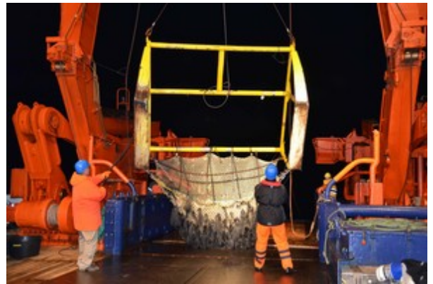
Fig. 5: The Agassiz Trawl comes on deck at night. (© A. Brandt)
