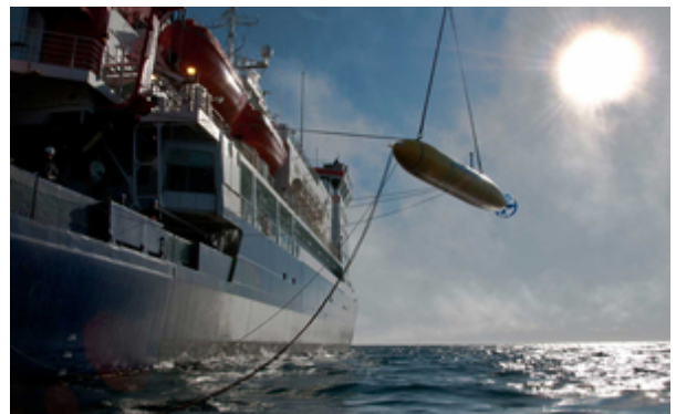
Deployment of the Autonomous Underwater Vehicle. (Photo: M. Ginzburg)
