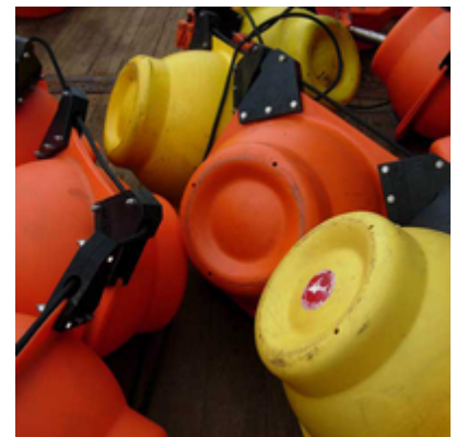
Fig. 2: Floats are needed to ensure the vertical orientation of the moorings in the water column.
