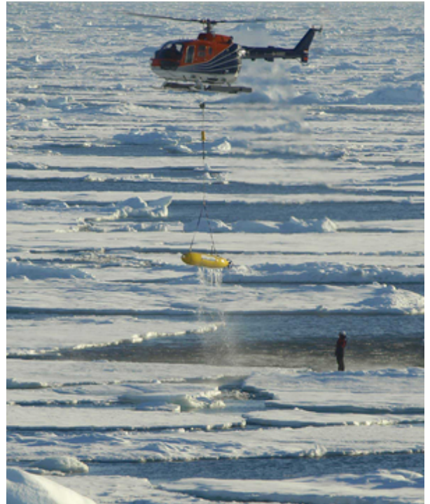
Recovery of the Autonomous Underwater Vehicle. (Photo: M. Jacob)
