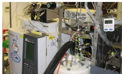
Gas chromatographic purge and trap system for a simultaneous measurement of SF6 and CFC-12 (© T. Stoeven, GEOMAR)
