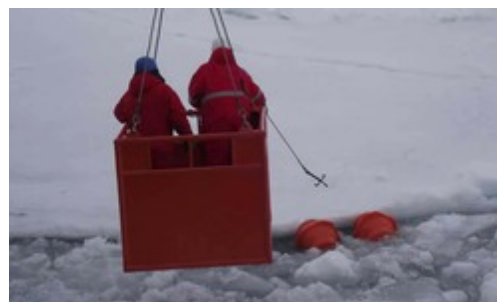
Fishing out the flotation balls from the person chair hanging on the crane after the mooring rope was broken. (© A. Beszczynska-Moeller/AWI)
