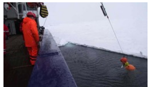
Pulling the top of the mooring from beneath the ice floe during recovery in ice (© A. Beszczynska-Moeller/AWI)
