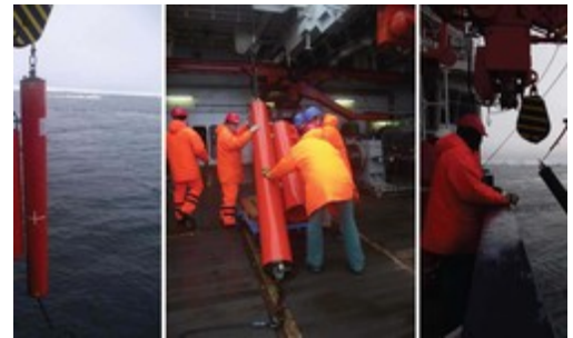
Recovery of moorings with different types of the acoustic RAFOS sound sources in the ice covered western Fram Strait (© A. Beszczynska-Moeller, AWI)
