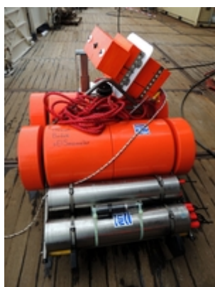
Figure 7 The ocean bottom SICEmometer back on deck after a first successful mission (Source: V. Schindwein AWI)
