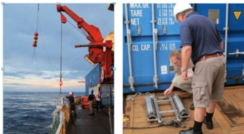
Pictures 3+4: Deployment of the Posidonia transponder. An old train wheel is used as an anchor weight (already below sea surface) and the orange buoys will give the transponder a lift from the sea bed to the water surface once released from the anchor (Pictures: S. Hanisch/AWI).
