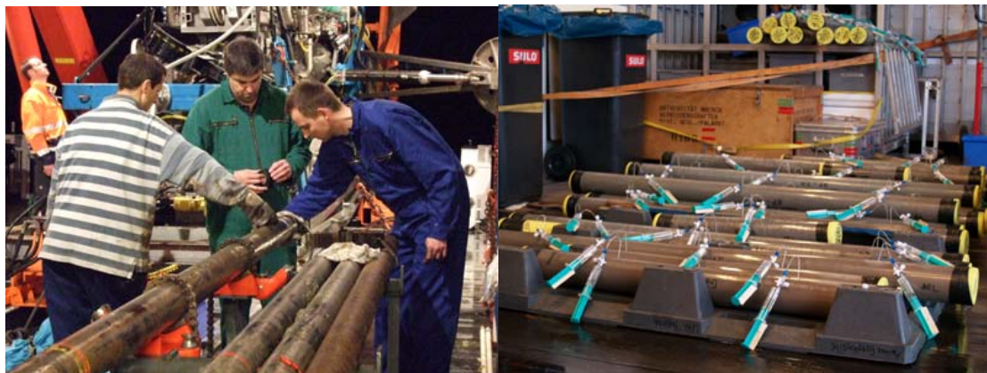
Left: Opening of the core barrels for recovery of the MeBo sediment cores; Right: pore water sampling using the suction method
