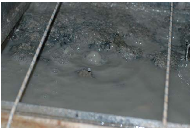
Fig. 2: "Boiling" water indicating the presence of gas hydrates in a box corer sample. Ten minutes after taken on board gas hydrates of substantial size were picked from the mud.
