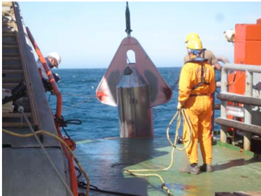
The PIG, the head system carrier of the HYDRA CSEM system returns on board.
