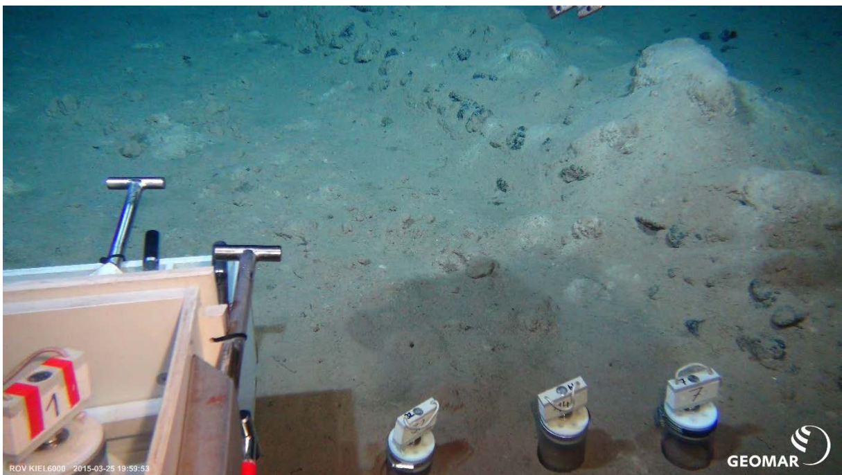
Beprobung mit den push-corers in der Spur. Sampling in the Track with the push-corers.
