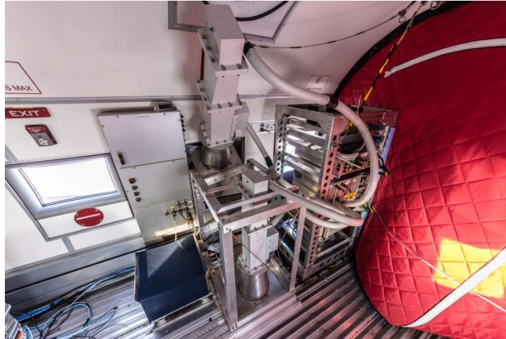
Figure 5: Installation of Nadir and Side-Looking EMIRAD-2 antennas in Polar-5
