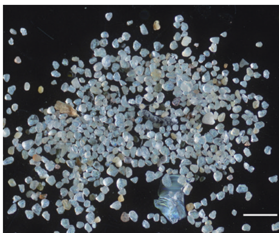
Fig. 8.2 Overview of a sample prepared for measurement by FPA-based micro-FTIR spectroscopy (sample WuKu_EU_04, scale bar: 1000 \mu\text{m} )
