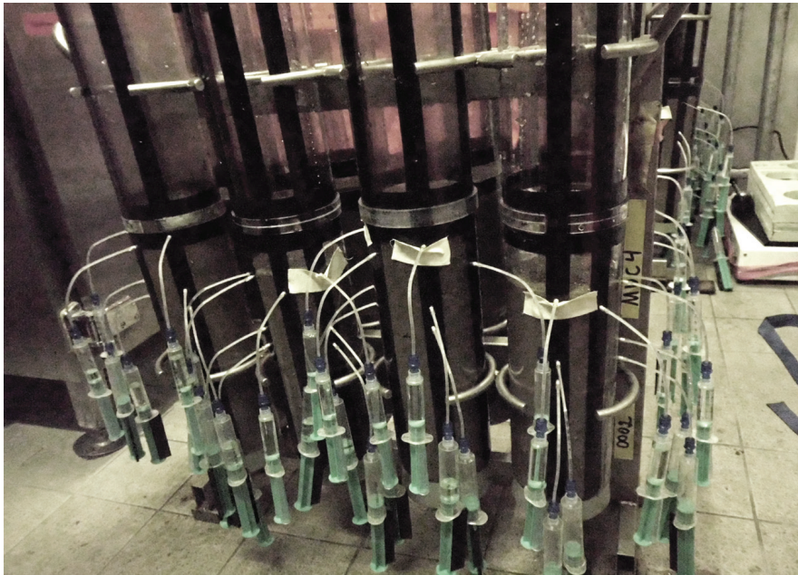
Fig. 3.1: Porewater sampling from sediment cores retrieved by a multiple corer
