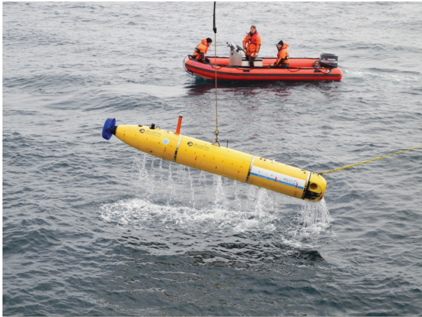
Fig. 6.1: Recovery of the AWI Autonomous Underwater Vehicle (AUV)
