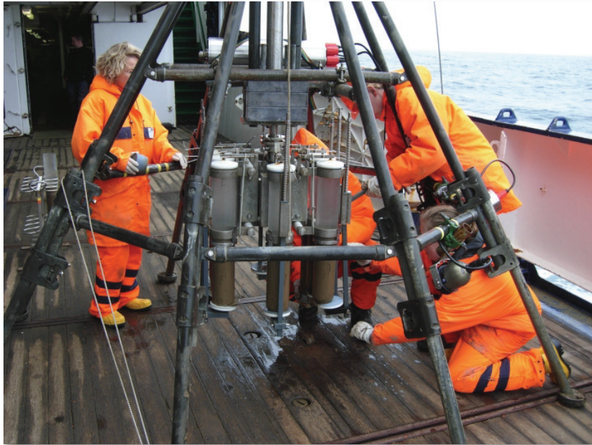
Fig. 2.3: Sediment sampling using a video-guided multiple corer (TV-MUC)
