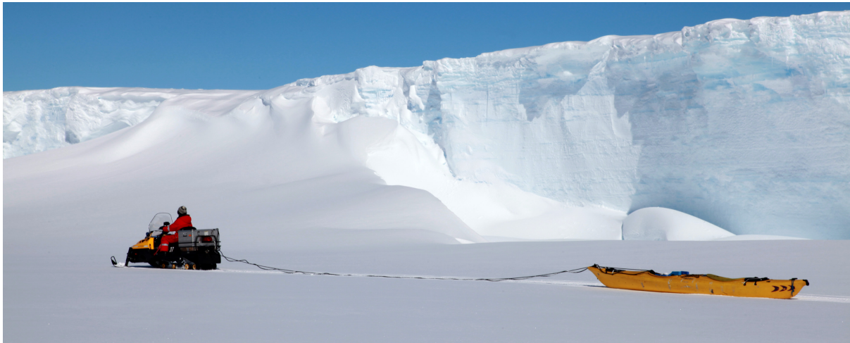
Figure 4.7: Kayak with EM31 pulled behind a snowmobile (photo by Jölund Asseng).
