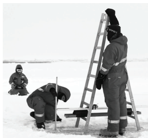
Fig. 2. Multi-frequency EM induction sounding data are recorded with the GEM-2 at different heights above sea ice. The signal directly depends on the distances to the conductive layers. Photograph by Sandra Schwegmann, 24 June 2013.
