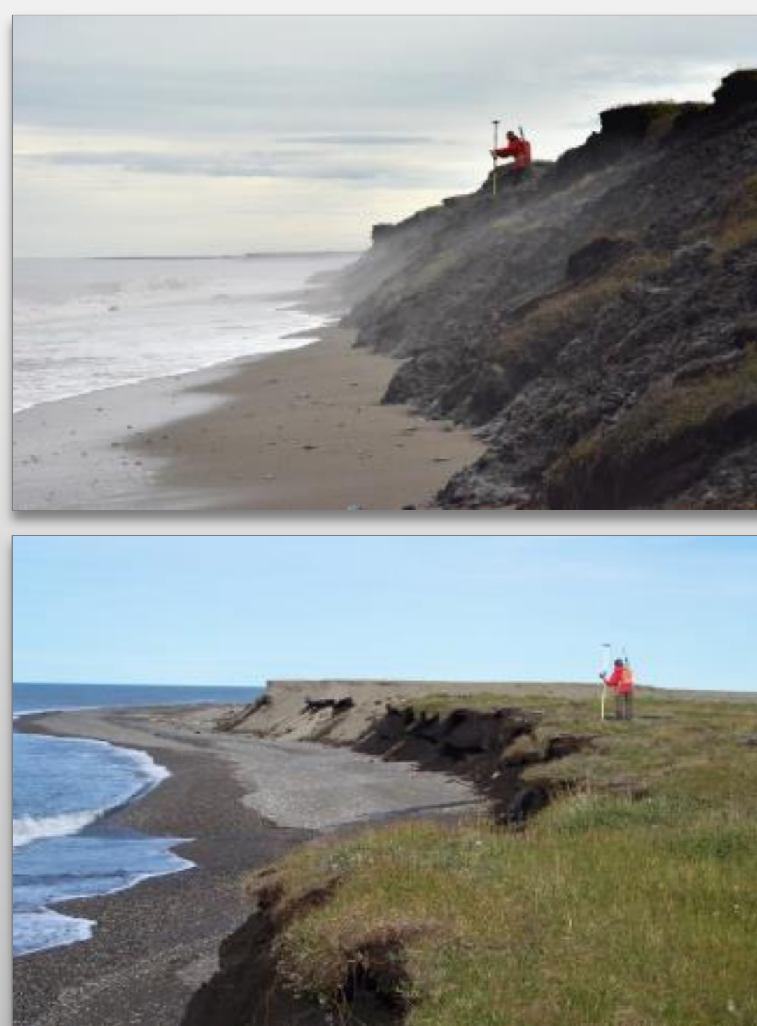
Figure 3: RTK-GPS measurements taken along the border site (top) and the Komakuk site (bottom) in 2012.
