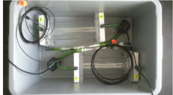
Fig. 8. Arrangement of the respirometers in the basin.
