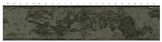
Fig.1: A scan of the sediment core GeoB20803-2 from a depth of 79 metres shows clear zones of disturbance caused by the gas dissolution.
