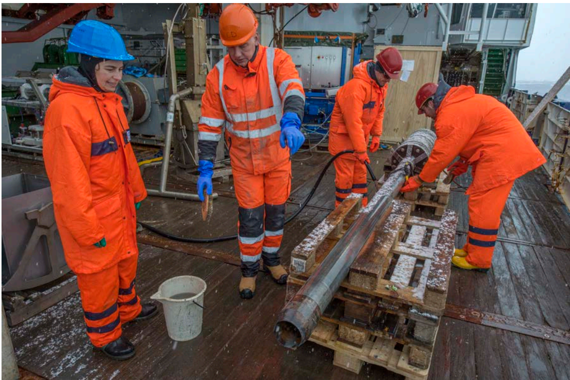
3 - The geologist explains to the biologist why the gravity corer only collected sea water – and why this is an important result. During past ice ages sediments on the Weddell Sea shelf were highly compacted when the Filchner-Ronne Ice Shelf grounded and advanced seaward. The seabed proves this by its refusal to provide a sample for the 1.5 ton weighing corer (Photo: AWI).
