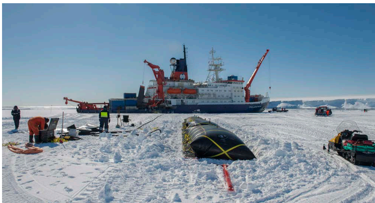
2 - Cargo unloading is carried out in front of the Rønne Ice Shelf under beautiful summer conditions with temperatures of -17\text{ }^{\circ}\text{C} . In the foreground you can see BAS fuel bladders on rubber mats that Pistenbulli tractors (background, right) will tow to their final destinations, such as ice-shelf drill sites ca. 500 km away. Photo: AWI.
