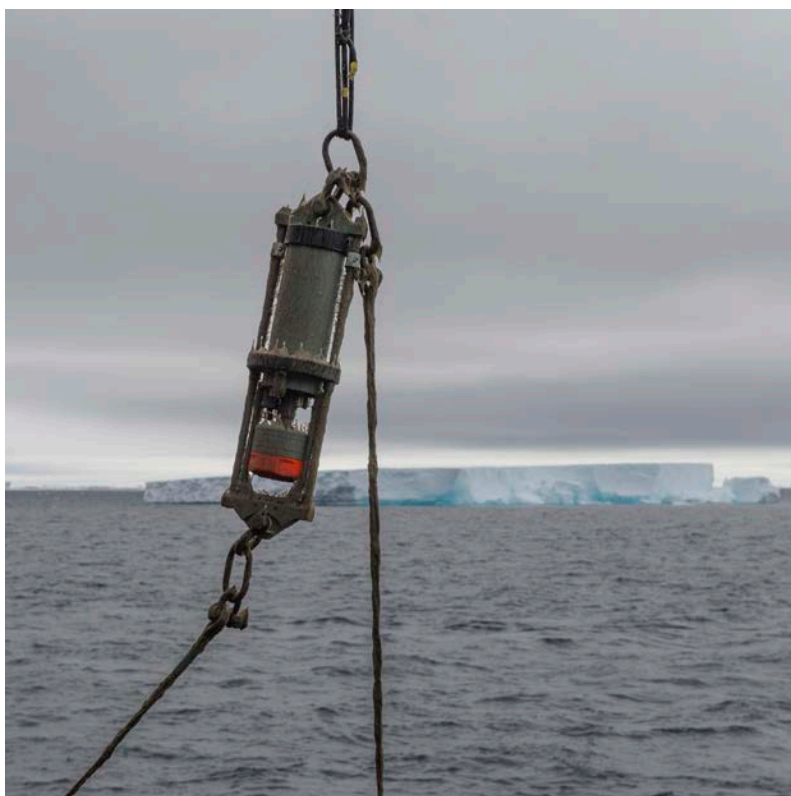
3 - A current meter in front of a tabular iceberg. This instrument was part of a mooring that measured for the last 2 years current direction and current speed of the bottom water flowing through Filchner Trough. In this photo, the current meter with its treasure trove of data is just being recovered and therefore shown upside down. The cylinder contains batteries, data storage and electronic components, while sensors (ADCP=Acoustic Doppler Current Profiler) are hidden under the red cap. Algae have utilised this hard ground for creating a "maritime meadow". Photo: AWI.
