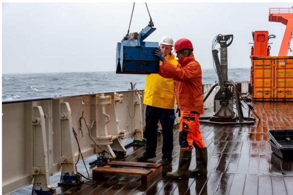
*The grab sampler is the most used device aboard the METEOR during the first week of the ATHENA cruise.*
