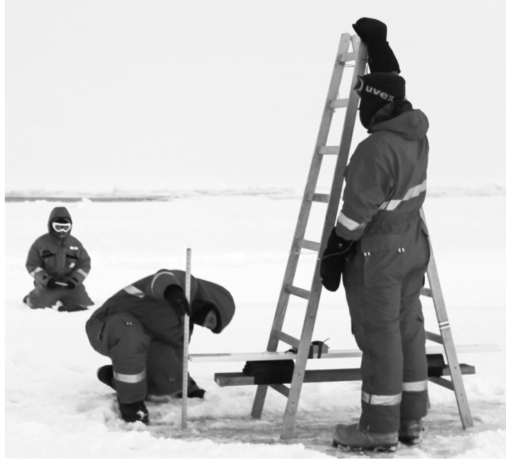
Figure 2.2.: Multi-frequency EM induction sounding data are recorded with the GEM-2 at different heights above sea ice. The signal directly depends on the distances to the conductive layers. Photograph by Sandra Schwegmann, 24th June 2013.
