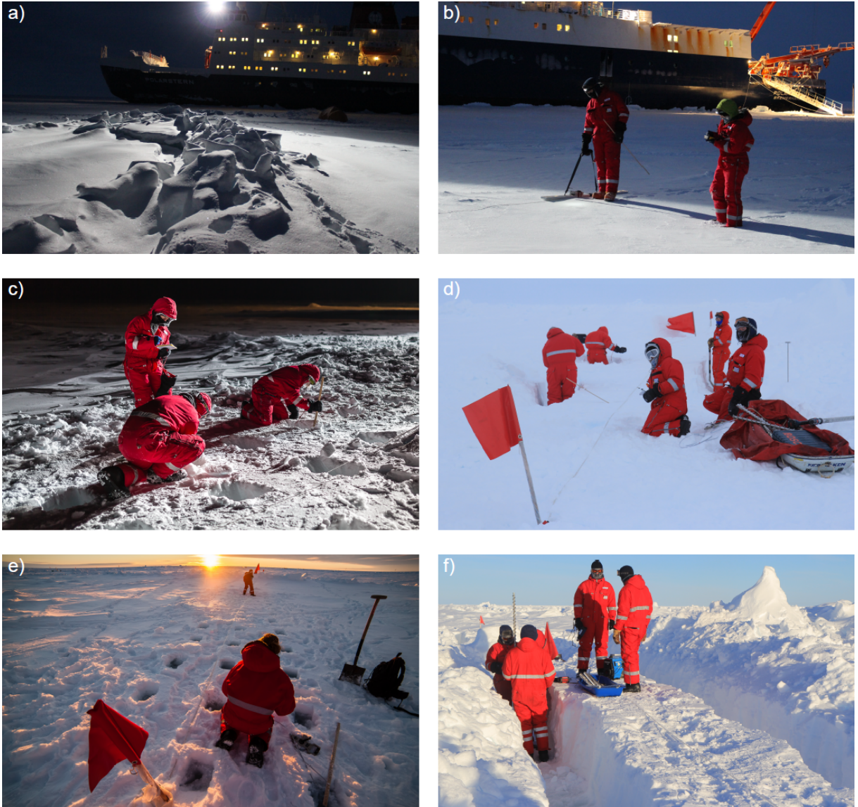
Figure 5.1.: Impressions of EM and validation measurements in the winter Weddell Sea, 2013. In a) a sea-ice pressure ridge is shown parallel to its sail and perpendicular to the transect, b) EM data were acquired with a GEM-2. c), d), e) and f) show validation measurements of snow thickness, sea-ice thickness, freeboard and voids between sea-ice blocks. Photograph credits belong of a) and b) to Sandra Schwegmann, c) to Stefan Hendricks, d) and f) to Bruno Jourdain and e) to Mario Hoppmann.
