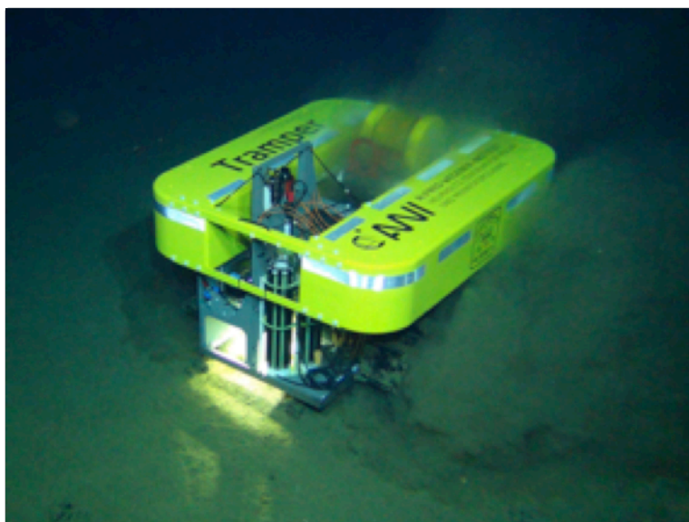
Fig. 5.4: The benthic crawler TRAMPER moving at the deep seafloor (© GEOMAR)
