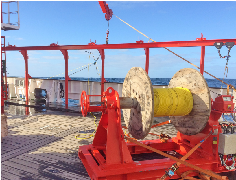
Fig. 6.3.1. The magnetometer cable was fitted to a mobile R/V Sonne winch for deployment off the port-side crane arm.
