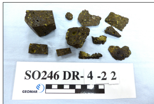
Fig. 6.7.5. Lithology 3 of DR04 at Pare Pekapeka guyot: highly vesicular lava with altered feldspar phenocrysts.
