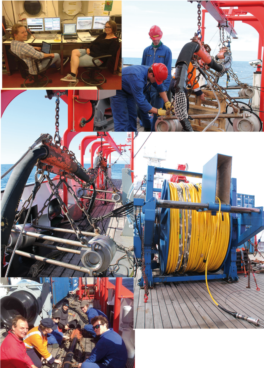
Fig. 6.2.1. G-Gun array and winch with streamer system on deck of RV Sonne. Seismic reflection team during airgun repairs and on watch in the seismic lab.
