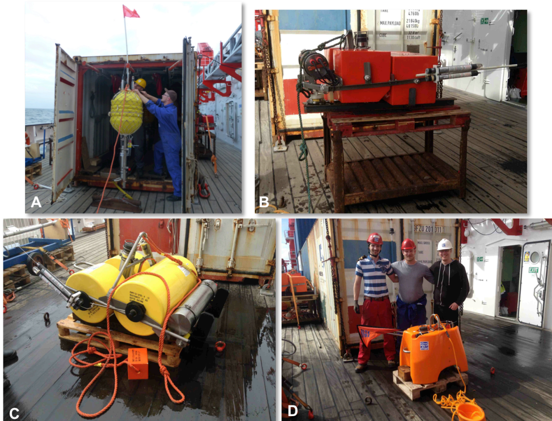
Fig. 6.2. Photos of the deployed OBS and OBH systems: (A) GEOMAR OBH, (B) GEOMAR OBS, (C) LOBSTER of AWI DEPAS pool, and (D) NAMMU prototype OBS of K.U.M. GmbH after first successful test.
