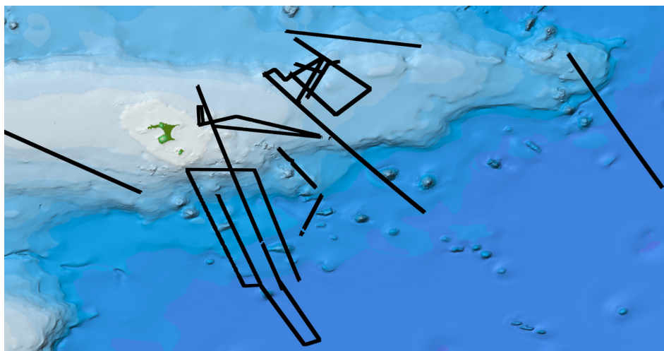
Fig. 6.3.3. Magnetic anomaly tracks from the SO246 survey plotted over bathymetry.
