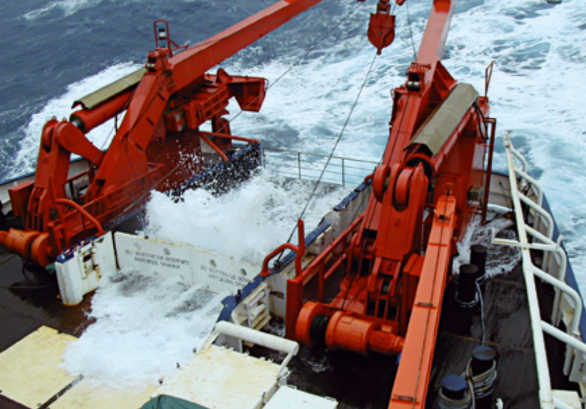
During an iron fertilization experiment in the Southern Ocean: To enable scientists to deploy the trace element iron, the RV 'Polarstern' is in an unfavourable position in the swells taking on a lot of water astern. Photo: AWI
