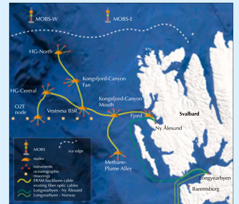
Schematic representation of the planned multidisciplinary FRAM (Frontiers in Arctic marine monitoring) observatory west of Spitsbergen. Autonomous measuring systems and new sensor packages are also installed as well as a satellite communications system that will allow real-time data transfer. Graphic: N. Lochthofen, AWI
