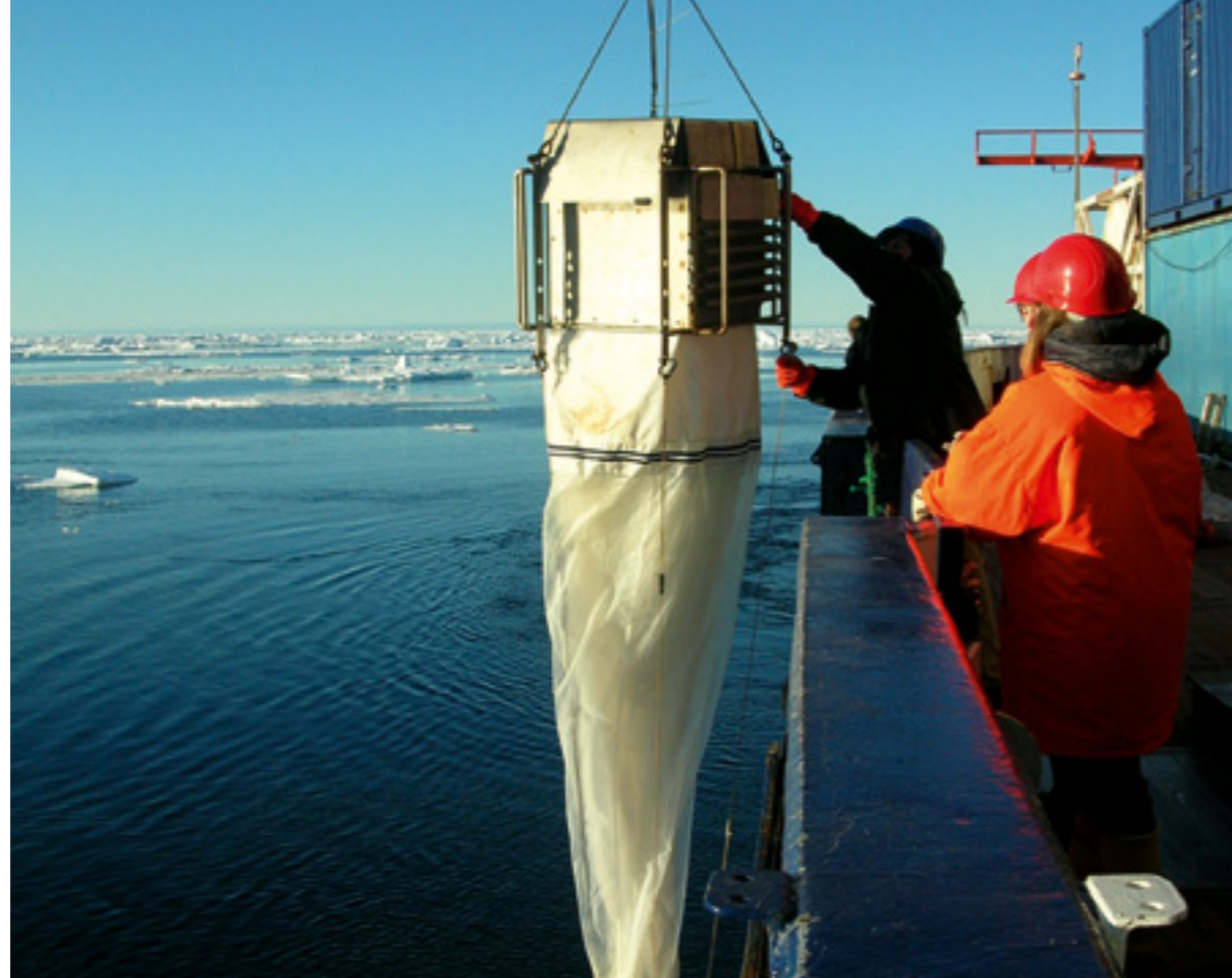
With the 'Polarstern' in the Arctic for a PhD: Plankton nets used during the expedition ARK XXV-2 to collect samples. Photo: V. Strass, AWI
