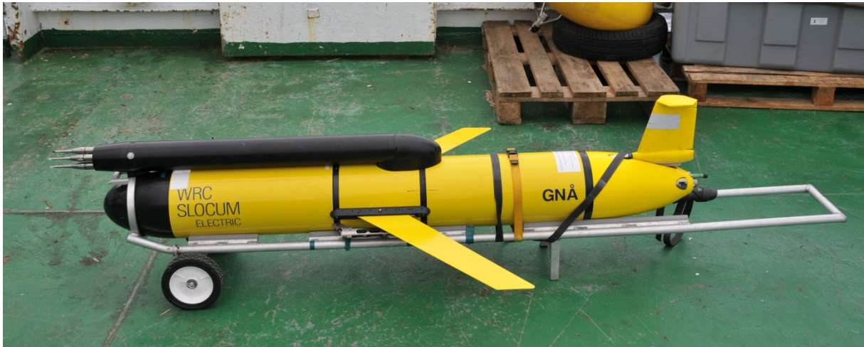
Figure 22. Photo of the glider Gnå mounted with MicroRider, strapped on the transportation trolley.
