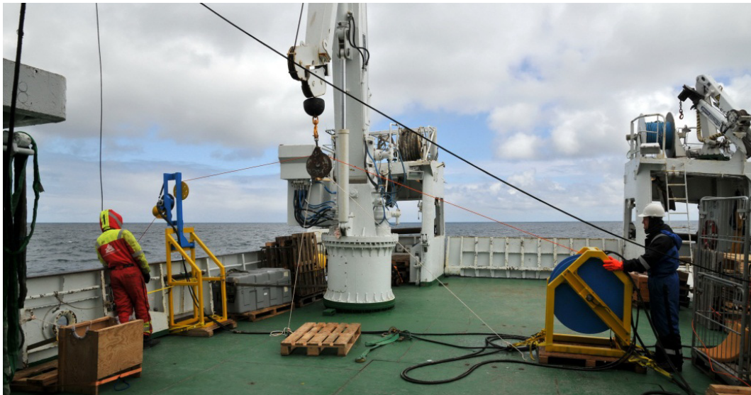
Figure 14. The set-up, on deck, of the VMP microstructure profiling system. The hydraulic winch is on the right; the cable is fed through a block supported by the crane in the middle. The block is fastened by ropes to the deck to avoid swings due to wind and ship's roll. The tether then is fed into the line-puller fastened to the ship's railing. In addition to the winch operator, a second person observes the cable in water during the deployment, and assists with deployment and recovery.
