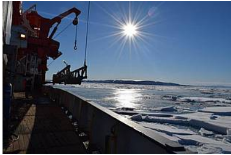
Fig.1: Gravity coring of marine sediments north of Norske Oer. (Photo: Alfred-Wegener-Institut)
