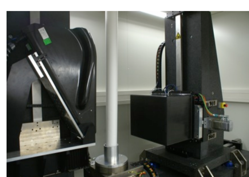
Figure 2: Setup of the AWI ICE-XCT (Freitag et al. 2013)
