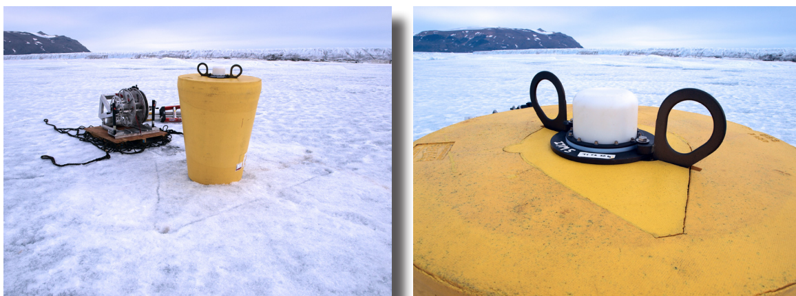
Fig. 3.7: Installed mooring. Surface package and winch at the mooring site (left). Detail of surface package mounted in float (right).
