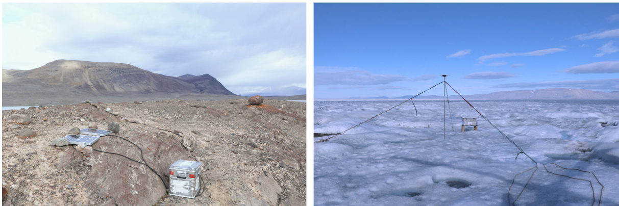
Fig. 8.1: Typical set-up of a GNSS station. Left: View at the final set-up of station CENT (Centrumsø). Right: At the glacier station NIOG (Nioghalvfjærdsbræ) the antenna is mounted on top of an iron rod fixed to the glacier by additional three guys. The solar panel is directly attached at top of the Zarges aluminium box.
