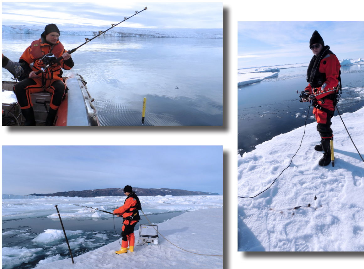
Fig. 3.6: Examples of usage of temperature-depth logger in the field. (a) Deployment from the zodiac. (b) Deployment from the side of an ice-floe. (c) After a deployment from the side of an ice-floe. The muddy lead weights are visible on the snow.
