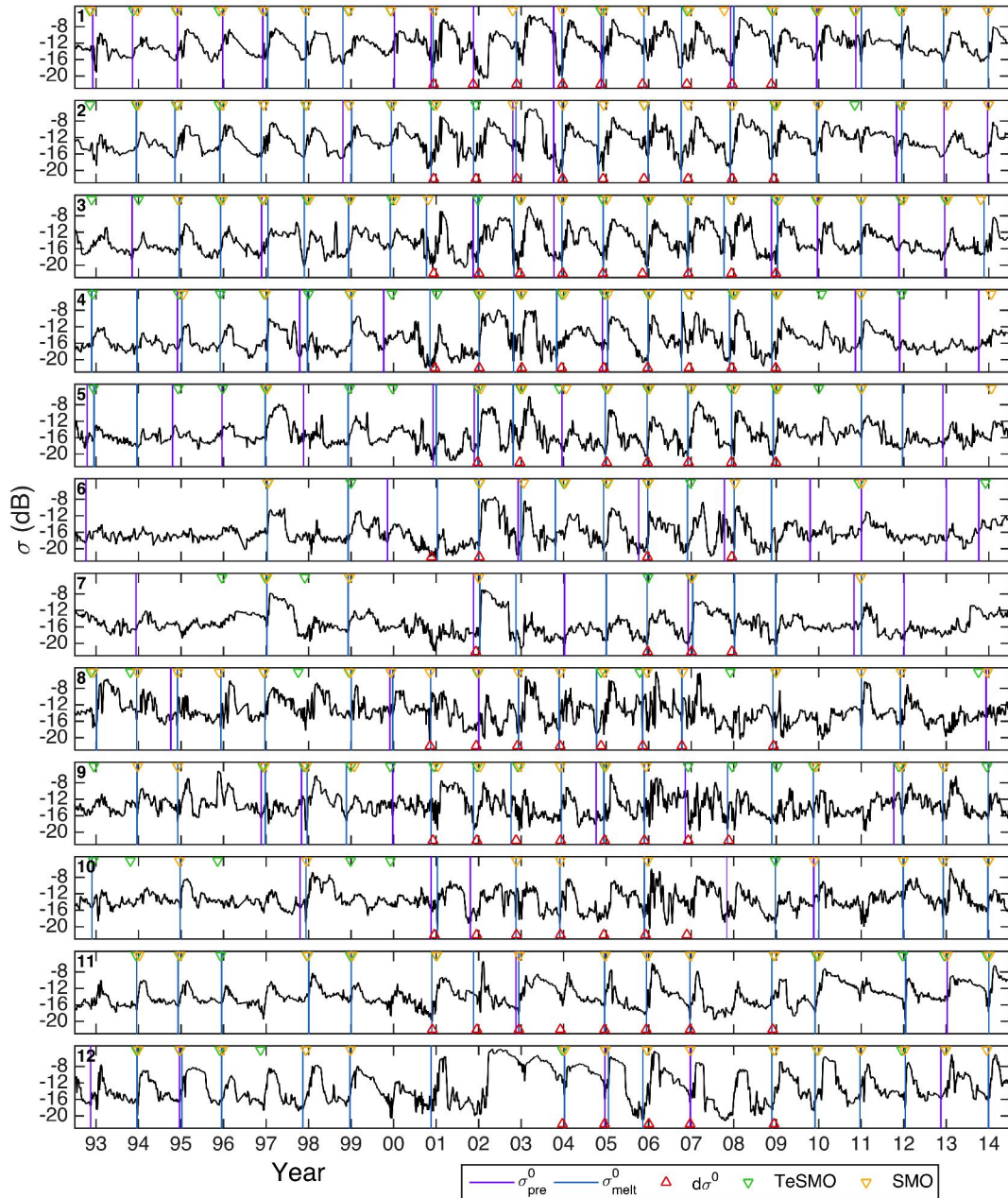
Figure 5.4: Time series of backscatter signals from 1992 to 2014 in the regions shown in Figure 5.1. The time series are composed from ERS-1/2, QSCAT and ASCAT data while from 2001 onwards the data are down-sampled to 6-day means according to the ERS data before. The purple and blue lines denote the snow pre-melt ( \sigma^0_{pre} ) and melt onset ( \sigma^0_{melt} ) retrieved from daily time series of \sigma^0 , respectively. The red triangle indicates the melt onset retrieved from its diurnal variations ( d\sigma^0 ). The green and yellow triangles denote the Temporary Snowmelt Onset (TeSMO) and Continuous Snowmelt Onset (SMO) from passive microwave observations according to Arndt et al. (2016).
