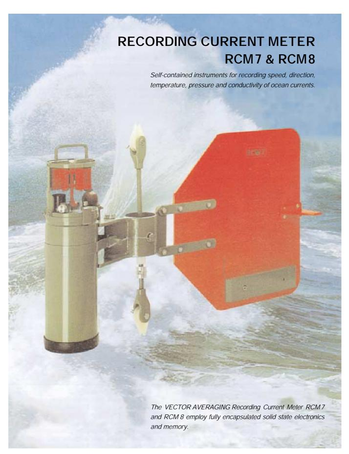
The measurement of ocean currents by a moored instrument is the standard method of obtaining information about the circulation of ocean waters. The RCM 7 is a self-contained instrument that can be moored in the sea and record ocean current, water temperature, conductivity of the water and instrument depth.
