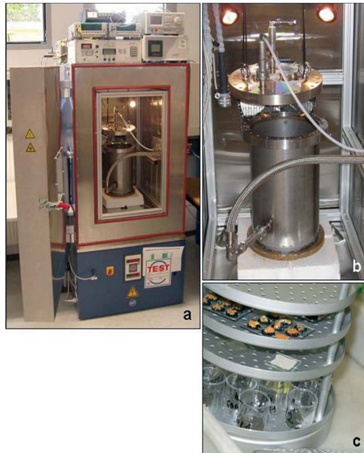
Figure 3. Mars simulation facility HUMIDITY- Lab for studying the effect of adsorption water on chemical and biological processes under the diurnal temperature and humidity profile of Mars. (a) cold chamber, (b) experiment chamber (c) rack for the exposure of biological samples.
