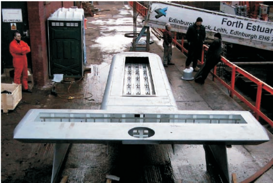
Figure 35 The blister for the EM 122 transducer arrays
