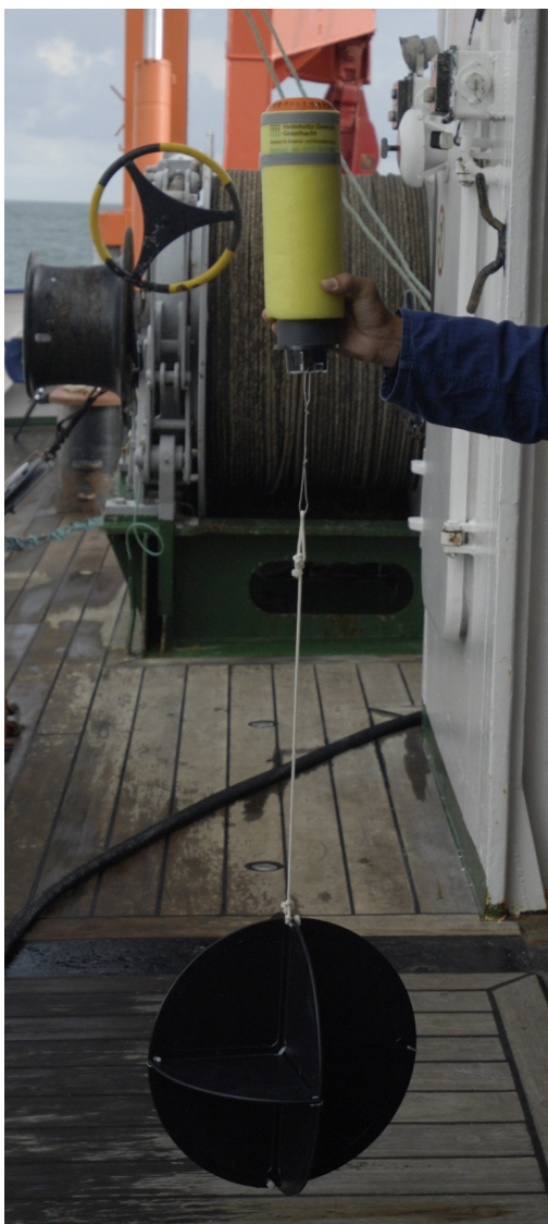
Figure 1: Drifters MD03i used during the experiment. The drifter sails were mounted 1.0 m under the sea surface and had a diameter of 0.35 m.
