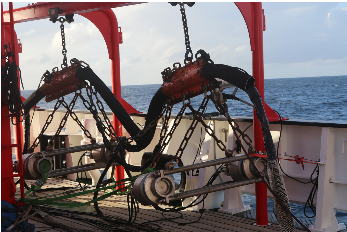
Fig. 5.2.3: G-Gun array used as seismic source. Photograph by Marc Hiller.
