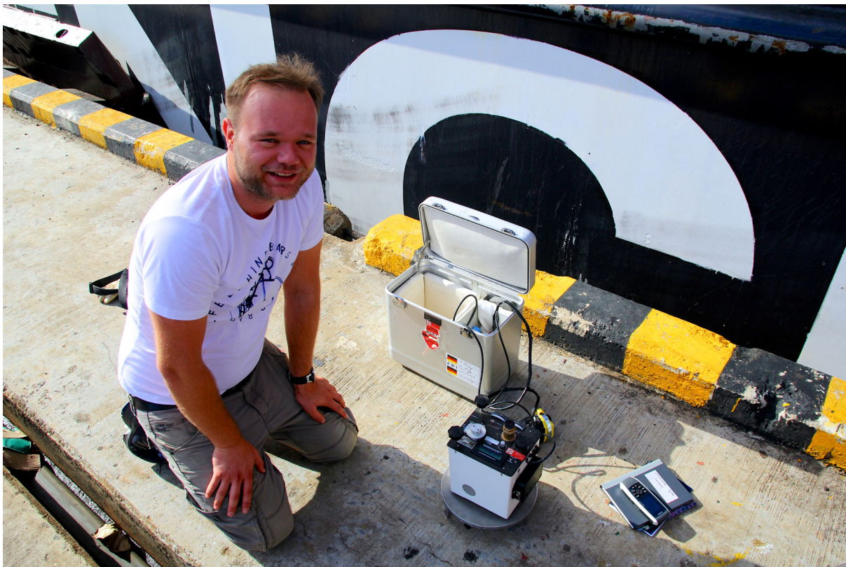
Fig. 5.4.5: Tie point measurement at the new North Pier in Colombo (#3).
