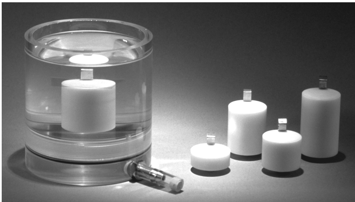
TEXT-FIGURE 1 Random settling device (left) and four slide carriers (right). The latter are used to attain different water column heights.
