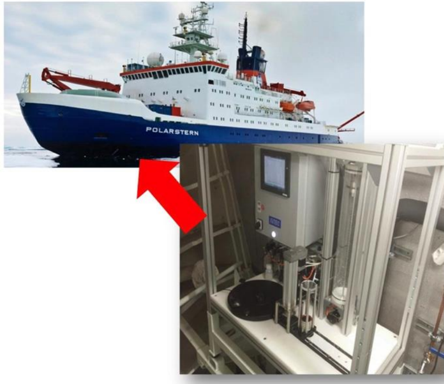
Fig. 5.1: The fully automated filtration module AUTOFIM is installed on RV Polarstern in the “Bugstrahlruderraum” close to the inflow of the ships-pump system. AUTOFIM is suitable for collecting samples with a maximum volume of 5 Liters. Filtration can be triggered on-demand or after fixed intervals. PHOTO: Katja Metfies
