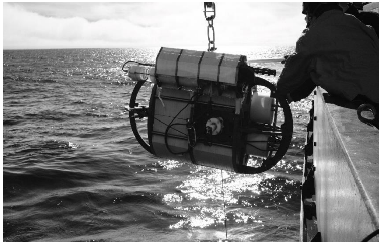
Fig. 2.4: Autonomous winch developed by technicians within the Deep Sea Ecology and Technology group in AWI, being deployed at HAUSGARTEN. These moorings winch throughout the year at programmed times to collect environmental information from the waters just below the sea ice, from regions where fixed moorings may be at risk. PHOTO: Mario Hoppmann
