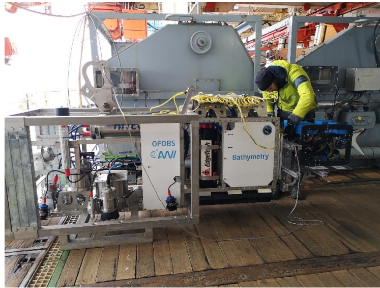
Fig. 2.2: OFOBS Camera sled, with miniROV mounted on the rear. This system will be used to both image and map regions of seafloor. PHOTO: Jannik Schnier
