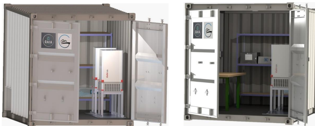
Fig. 6.1: Project rendering of GAInfrA, with the low-volume samplers in the foreground (only a few examples of the available instruments are depicted, a full list is reported in the text).
