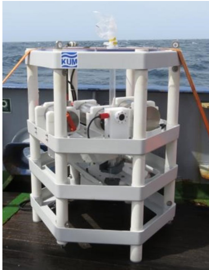
Fig. 4.10 The Bio-Optical Platform was developed by the SeaPump group at AWI and MARUM and measures size-specific settling velocities of organic aggregates two times daily during a one-year deployment. Additionally, it collects intact and individual aggregates in 40 gel traps, which each is open between three and seven days.
