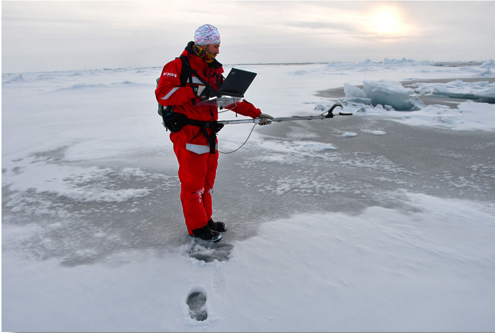
Fig. 2.3: Measuring spectral albedo using the ASD spectral radiometer at ArcWatch-1 station ICE 9.
