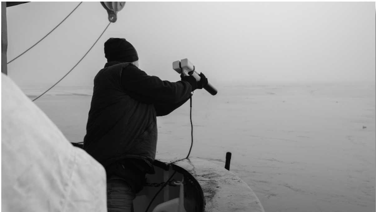
Fig. 3.4: XCTD deployment using a hand-held launcher
