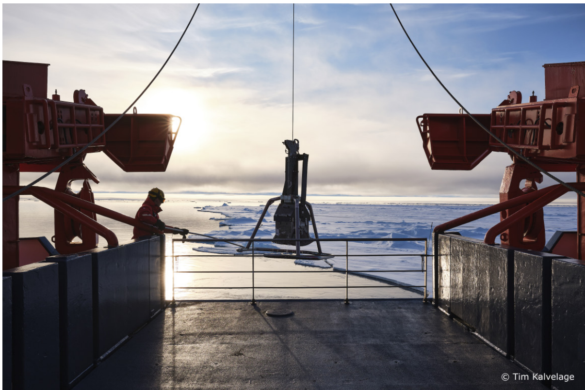
Fig. 5.3.1: The Giant Box Corer back on deck after successful deployment from the aft of the vessel.
