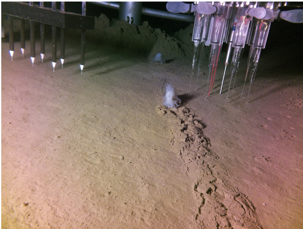
Fig. 5.5.2 and fiberoptical profiler (right) and deep profiler (left) recording in-situ profiles at station Ice-6 (PS138_136-1)
