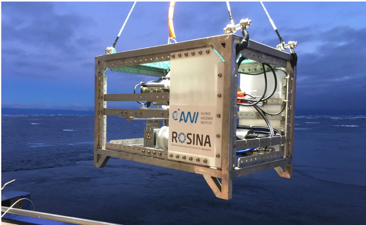
Fig. 4.8: ROSINA frame with the ROSINA camera system, Jelly camera and the Idronaut CTD
