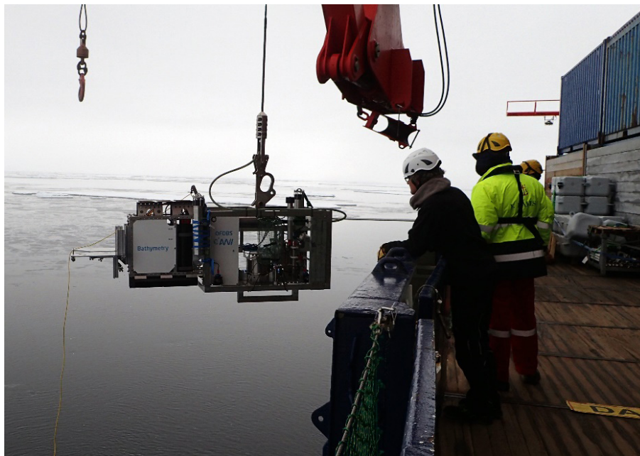
Fig. 5.2.1: Ocean Floor Observation and Bathymetry System (OFOBS)
