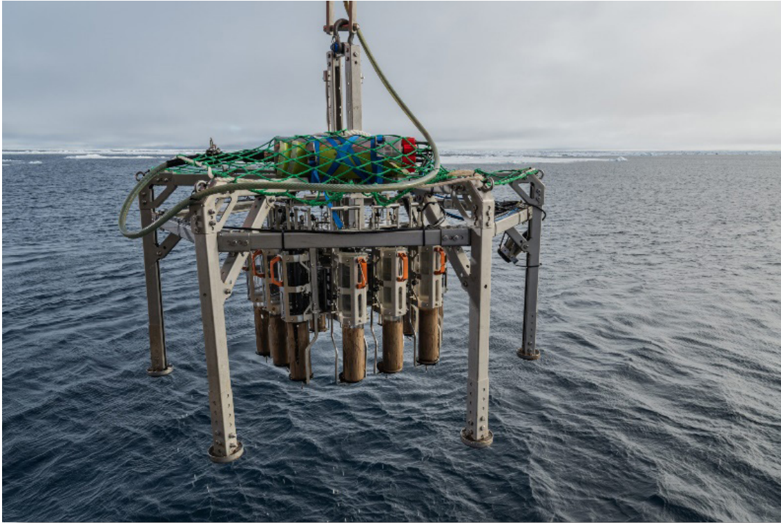
Fig. 5.4.1: TV-guided Multicorer (TV-MUC) with 12 sediment cores. © Esther Horvath
