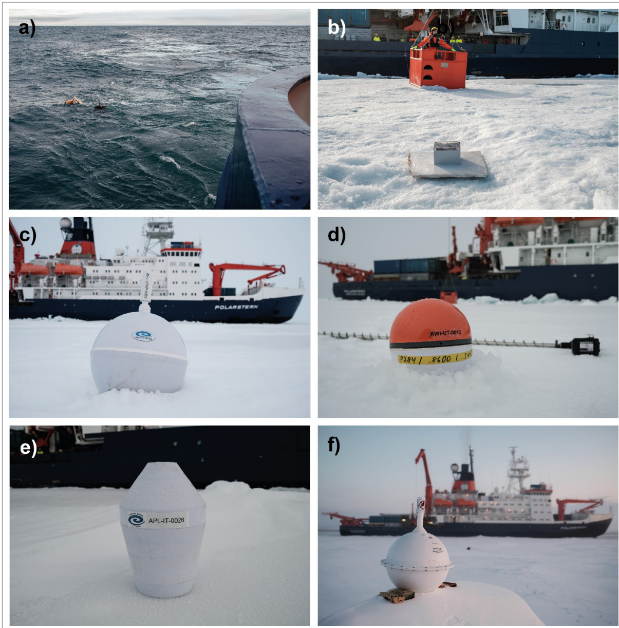
Fig. 6.3: Overview of different GPS buoys deployed during transit: a) NKE Trusted Buoy 2023P270; b) OpenMetBuoy 2023X16; c) Pacific Gyre Universal Tracker 2023P288; d) Pacific Gyre Universal Tracker 2023P284; e) Pacific Gyre Ice Tracker 2023P289; f) MetOcean SVP-B 2023P267
