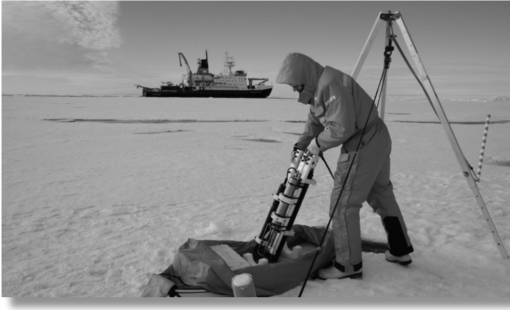
Fig. 3.7: Photo of ice-based SUNA nitrate profiling setup.
