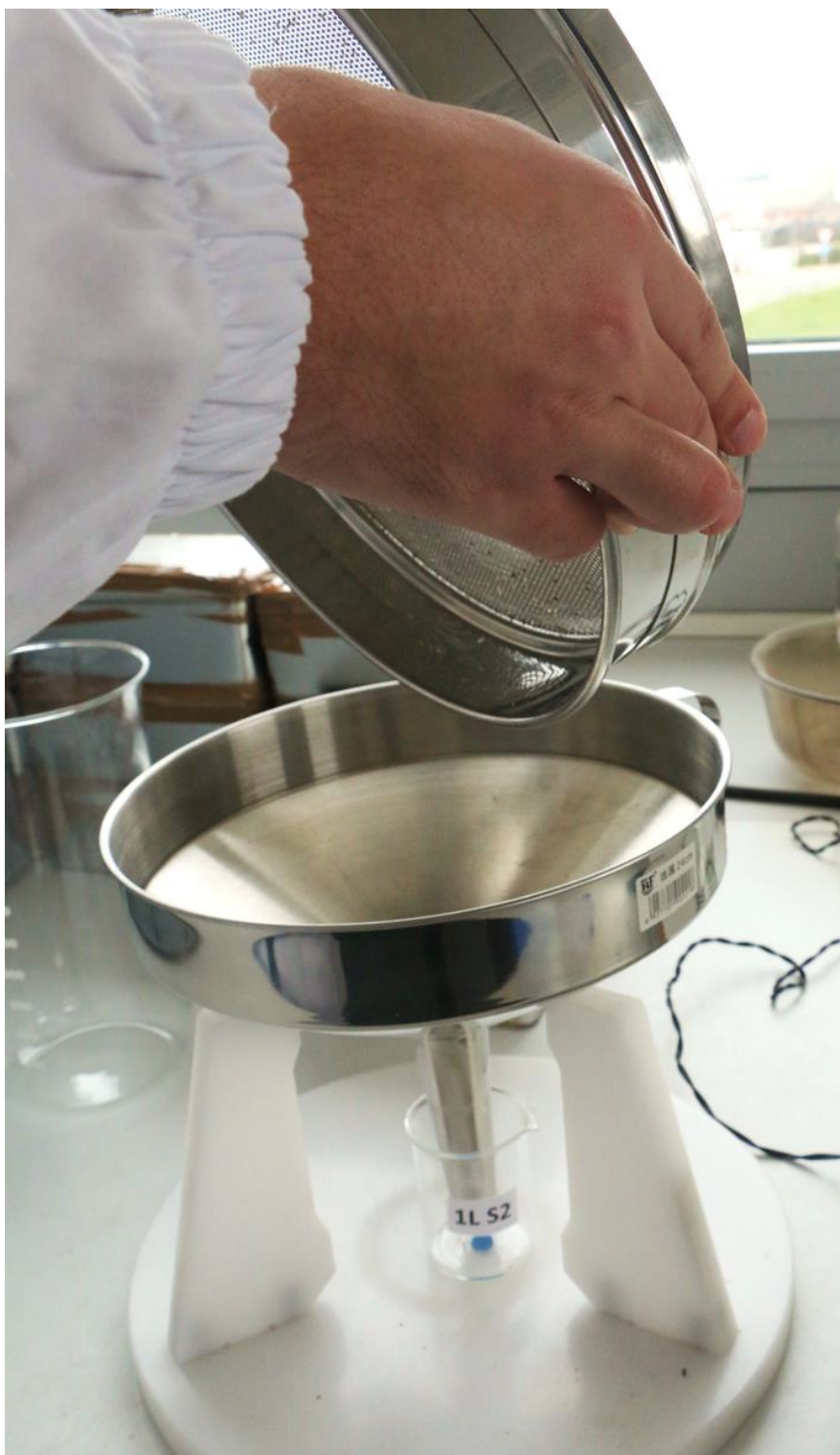
Figure S9. Transferring the contents from the 1-mm sieve through the metal funnel into a labelled small glass beaker.
