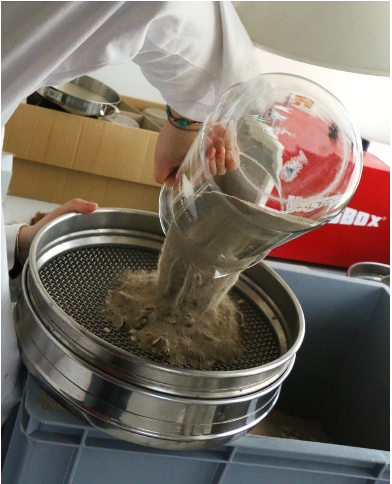
Figure S7. Pouring the sand sample from the volume beaker through the 5-mm sieve on the top and the 1-mm sieve at the bottom with any material passing both sieves caught in a large box.
