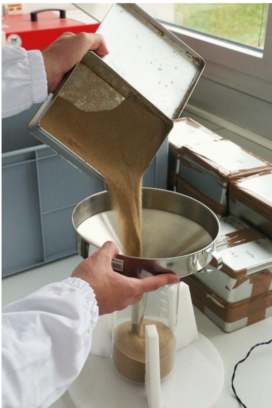
Figure S6. The contents from one sampling container were poured into a volume glass beaker through a metal funnel. The volume glass beaker was held in place by a specially built holder so that the glass beaker could not fall over.
