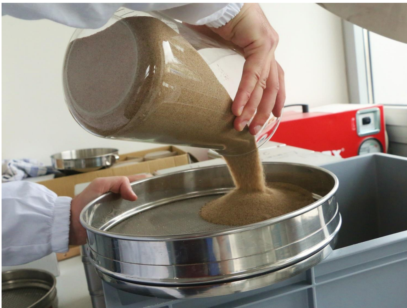
Figure S8. Pouring the sand from the volume beaker through the 1-mm sieve with any passing material caught in a large box. The red DustBox is visible in the background.
