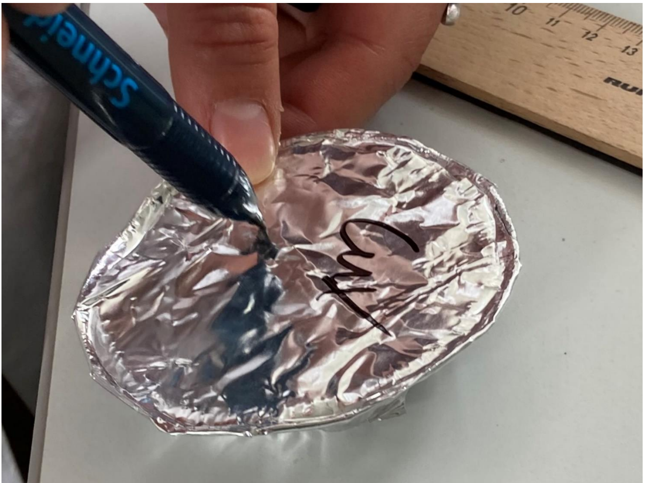
Figure S5. Sealing and labelling the aluminium cup containing the 50 g subsample for the sand grain size analysis.
