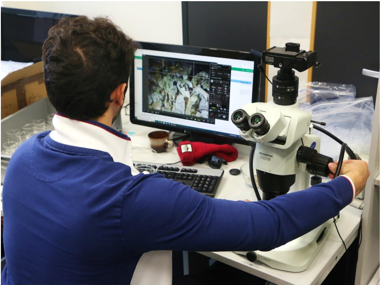
Figure S12. Our photo setup consisted of a binocular microscope with 2x or 5x magnification with an Olympus digital camera placed on top. The camera took photos (e.g., Figures S13-S14) via a computer using the OM capture software ( https://app.olympus-imaging.com/olympuscapture/ ).
