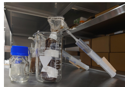
Figure 2.2: Setup to extract pore water from peat samples with Rhizons
