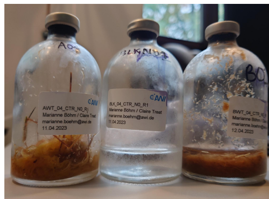
Figure 2.4: Examples of incubation vials of peat from above (left) and below the water table (right), and a procedural blank (center).
