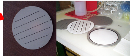
Single stage impactor with a cut off diameter at 2 µm (left) and silicon oil covered cellulose filter as well as a backup filter (right)
