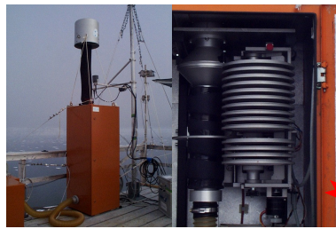
High-Volume aerosol sampler (left) and automatic filter changer with 15 single stage impactors (right)
