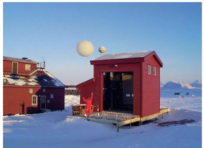
Fig. 4: Launch of an ozone sonde from the balloon house. Photo: R. Neuber.
