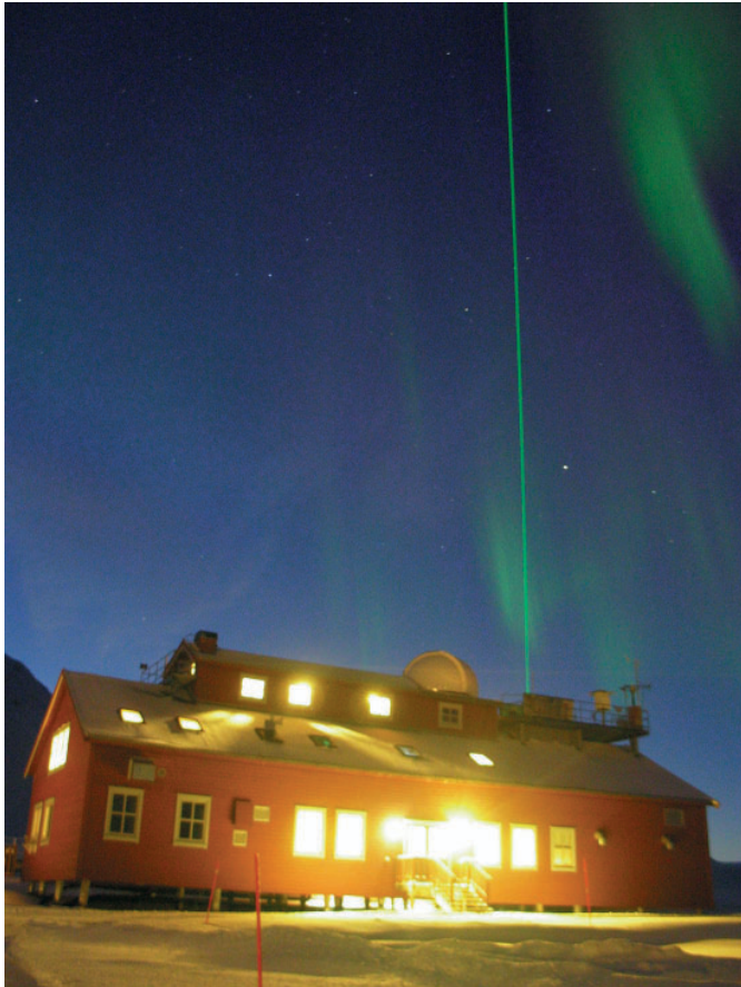
Fig. 3: The atmospheric observatory during the polar night. With the green laser beam the altitude distribution of aerosols and Polar Stratospheric Clouds (PSCs) are determined. Photo: R. Neuber, 2003.
