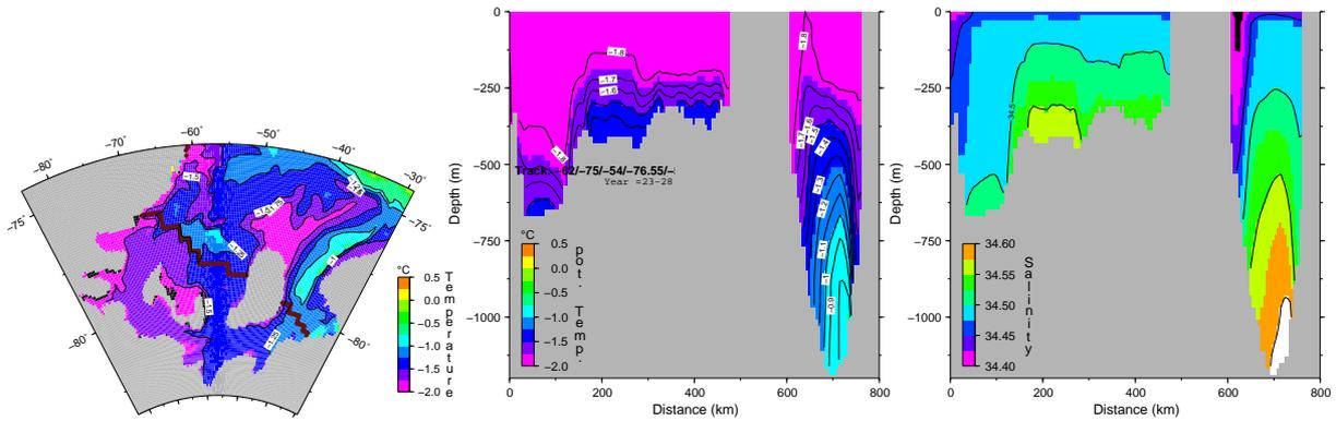
Figure 7: Bottom layer temperature (left), and temperature (middle) and salinity (right) cross sections along the track shown in Figure 1 for the scenario  $\mathcal{S}_{EF}$ .
