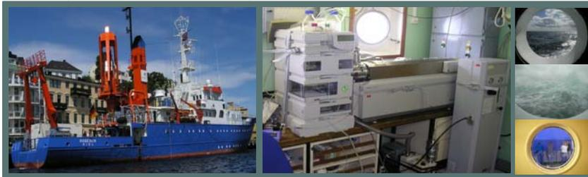
An API 4000 QTrap LC-MS/MS system on board the research vessel FS Poseidon
