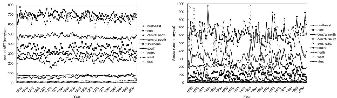
Figure 3. Dynamic changes of water fluxes in different rivers and watersheds during 1901-2002: (a) mean actual evapotranspiration and (b) mean runoff. Data were averaged over the regions.
