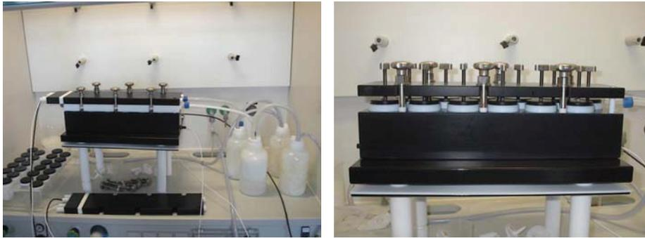
**Figure S 1:** left: *Experimental setup for pre-concentration of liquid samples before the addition of acids and after acid digestion.* Right: *Experimental setup for the acid digestion of Antarctic ice core samples.*
