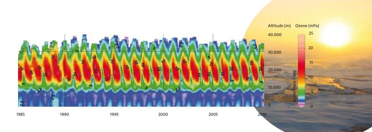
As shown in Figs. 1 and 2, the dramatic ozone depletion is restricted to certain altitudes (15 to 18 km) and seasons. In the last 25 years the mean ozone partial pressure in the Antarctic spring (September to November) has declined (Fig. 3). Whereas the mean values for the ozone layer were around 6 mPa in the 1980s, only half of that has been measured in recent years. At the same time the temperature at this altitude and in this season also changed.
