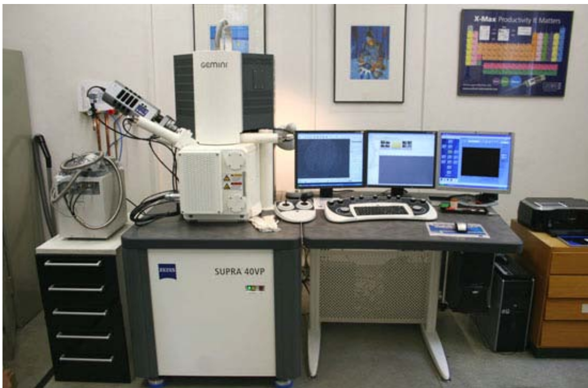
Figure 8: SEM aperture located at the Paleontology Department of the Freie Universität, Berlin (courtesy: J. Evers).
