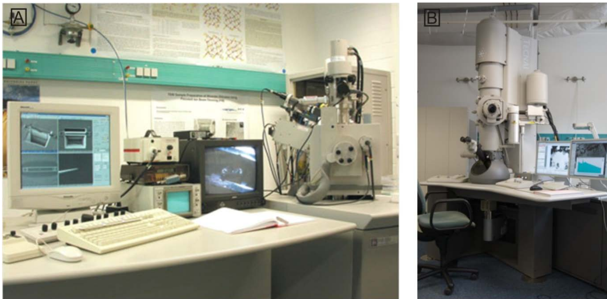
Figure 7: (A) Sample preparation using a FEI FIB200TEM. (B) A FEI Tecnai™ G2 F20 X-Twin with a HAADF Detector has been used for visualizing microstructures on quartz. (Both pictures are the courtesy of the GFZ Potsdam.)
