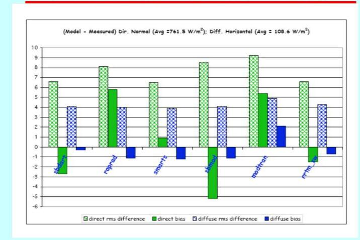
The above shows the biases (solid color) and RMS (cross-hatch) differences between various model calculations (as indicated) and observations for a multi-day period where the observed atmospheric states and composition were incorporated into the models. Michalsky et al. 2005.
