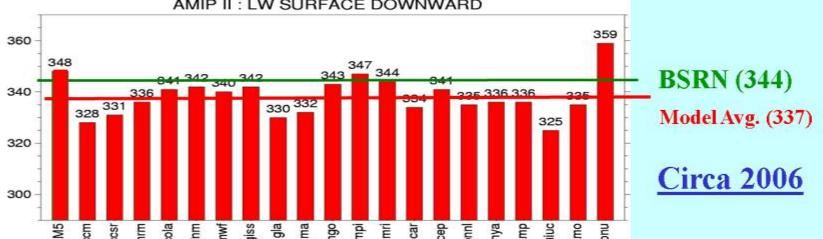
The above two graphs show global mean downwelling surface IR irradiance from numerous GCMs as indicated. The top plot shows results for the models from the mid 1990s whereas on the bottom plot are results about a decade later with the differences due to model changes and improvements. The green horizontal line is the global mean value deduced from BSRN data from site-by-site comparisons to a GCM, M. Wild, J. Clim. 2001 & Tellus 2008.
