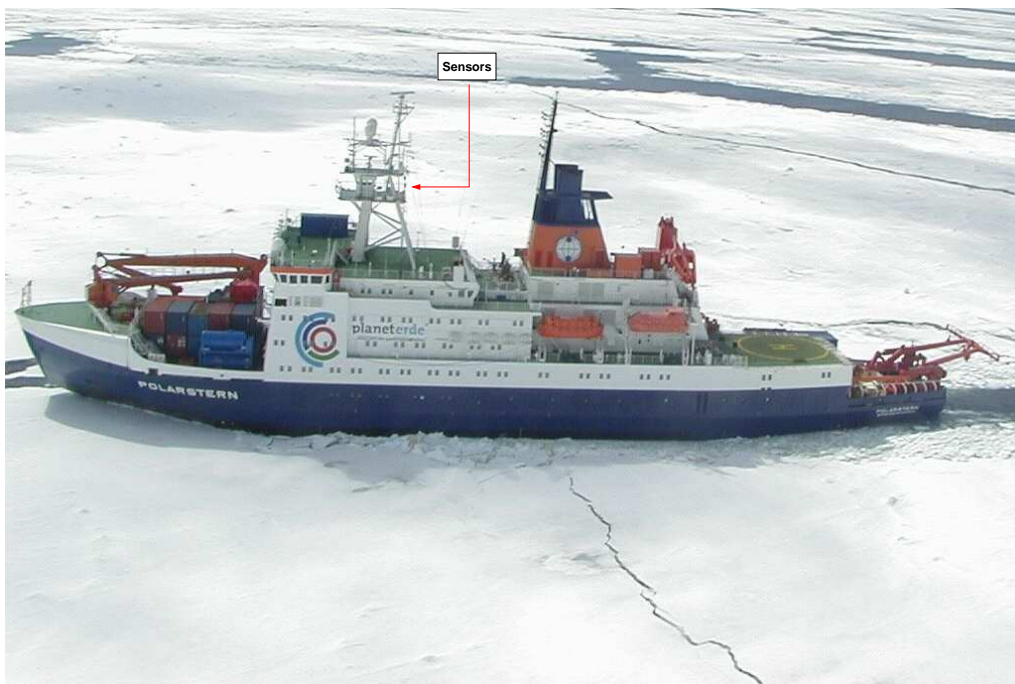
Figure 2.3-2: Overview of RV Polarstern . The magnetometer sensors are mounted astern on the main platform of the crow's nest as indicated.
