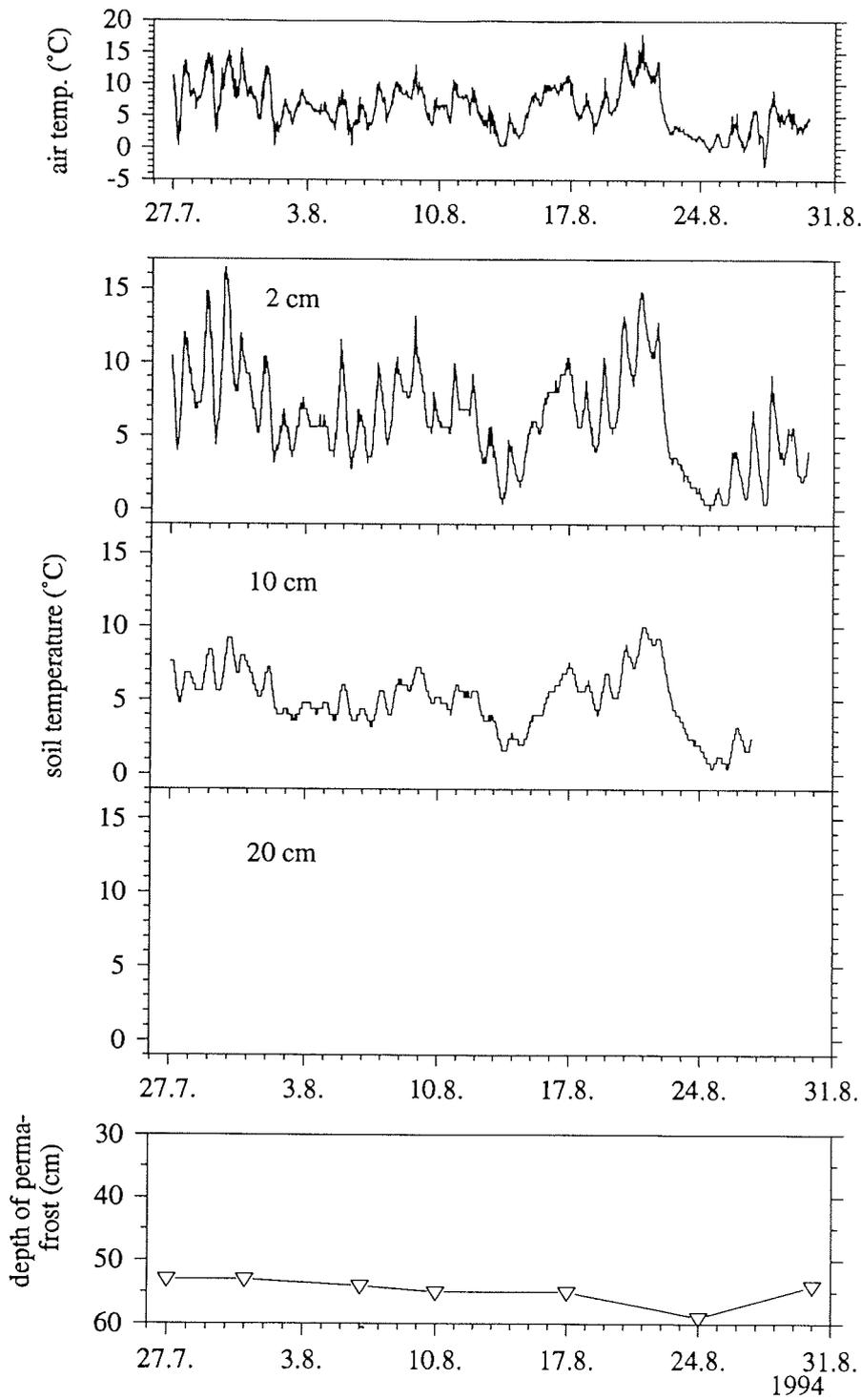
**Figure 3.10:** Ambient temperature, soil temperatures and depth of permafrost in humid tussock tundra, tussock.
