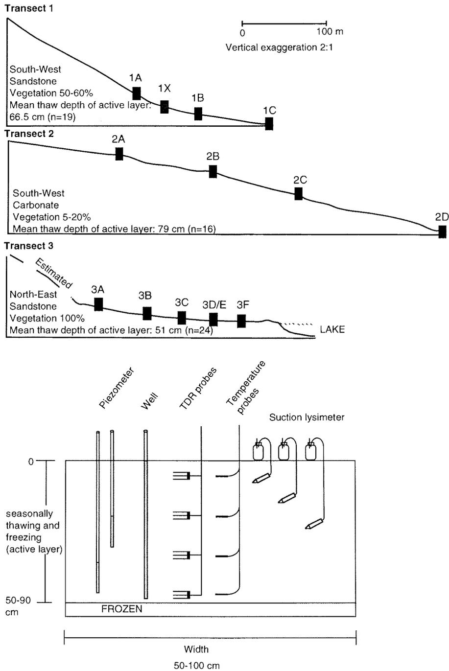
**Figure 2.11:** Cross section of transects and schema of instrumented soil pit
