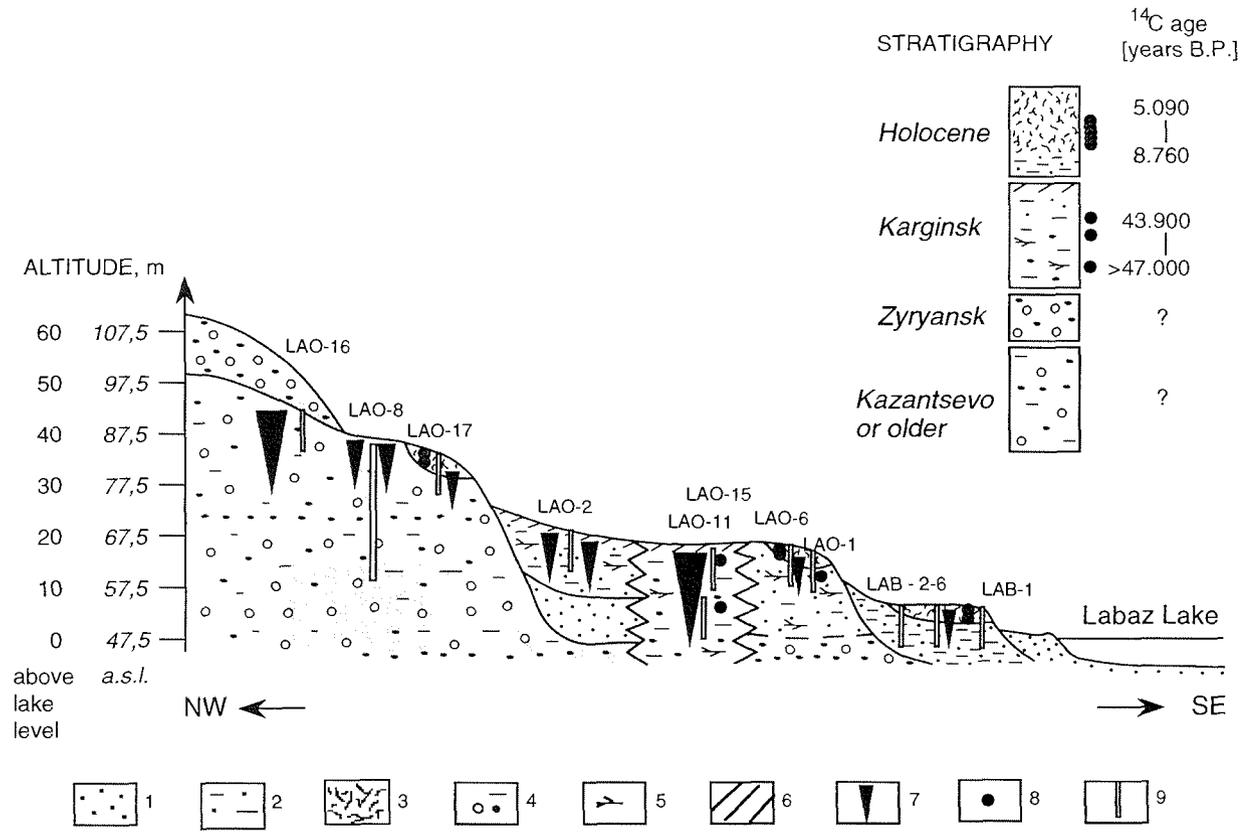
**Figure 3.2:** Schematic section and stratigraphy of Quaternary deposits in the northern shore zone of the Labaz Lake
