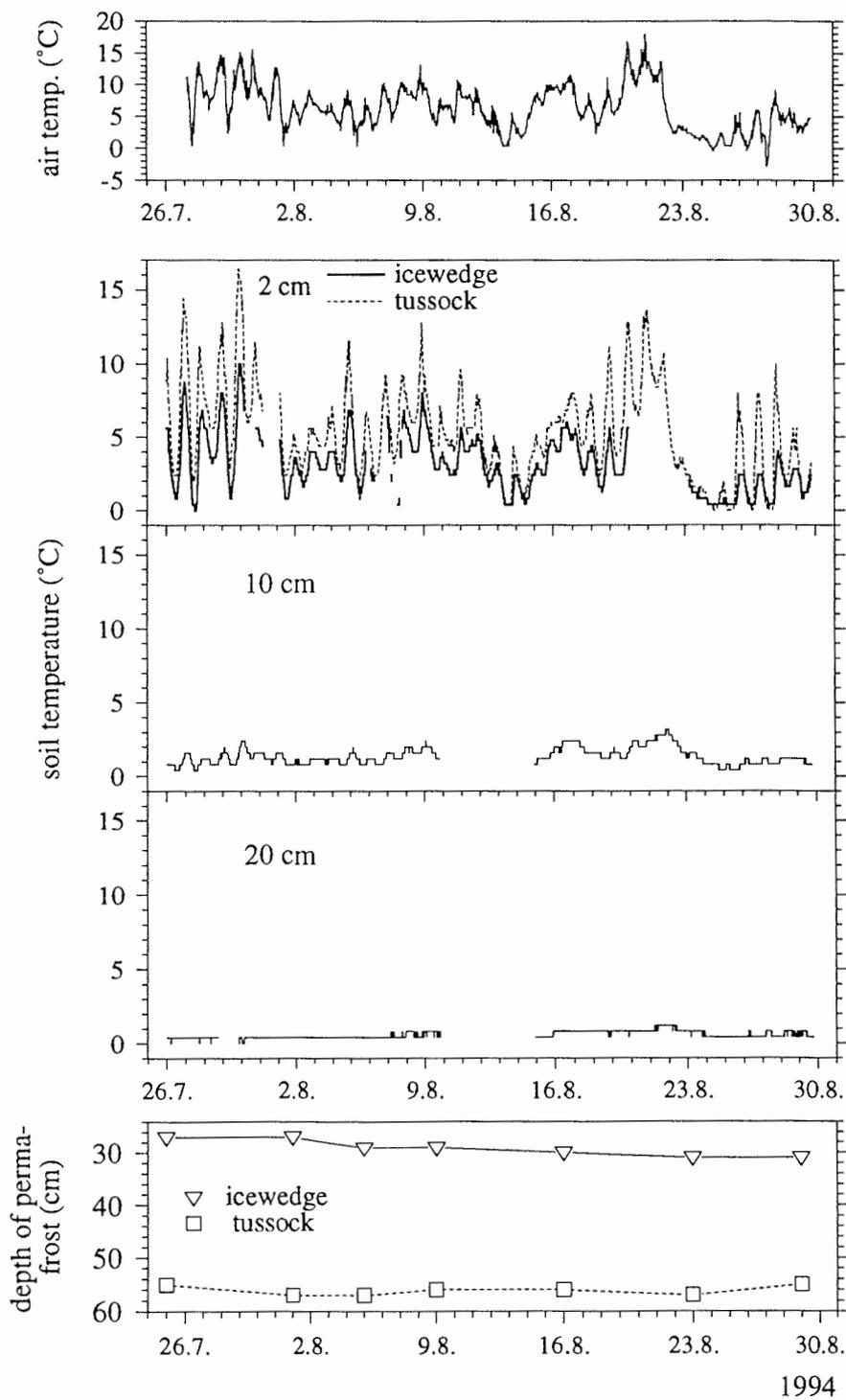
**Figure 3.9:** Ambient temperature, soil temperatures and depth of permafrost in mesic spotty tundra.
