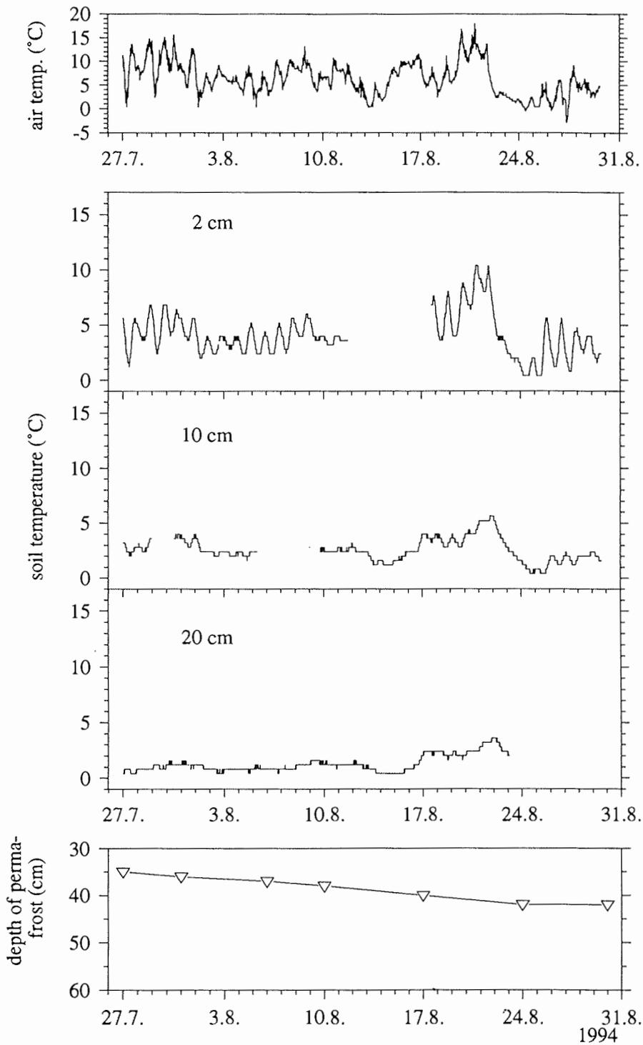
**Figure 3.11:** Ambient temperature, soil temperatures and depth of permafrost in humid tussock tundra, ice wedge.
