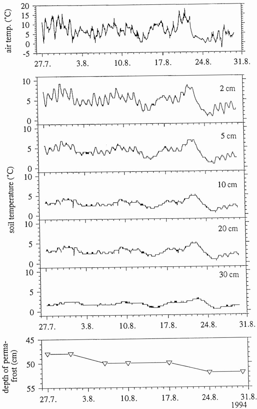
**Figure 3.12:** Ambient temperature, soil temperatures and depth of permafrost in wet sedge tundra.
