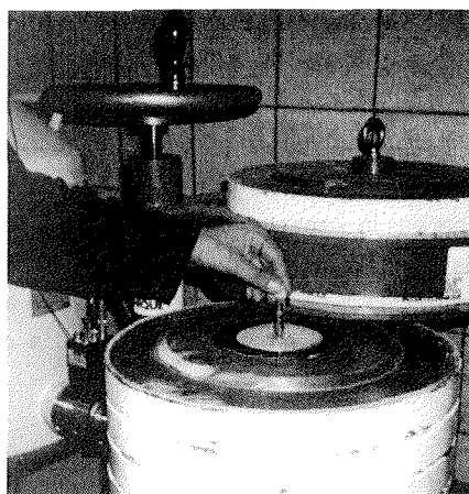
Fig. 18: Insertion of a sample in the borehole detector of a \gamma -spectrometer. The detector is surrounded by a lead shield from all sides to reduce the background radiation.
