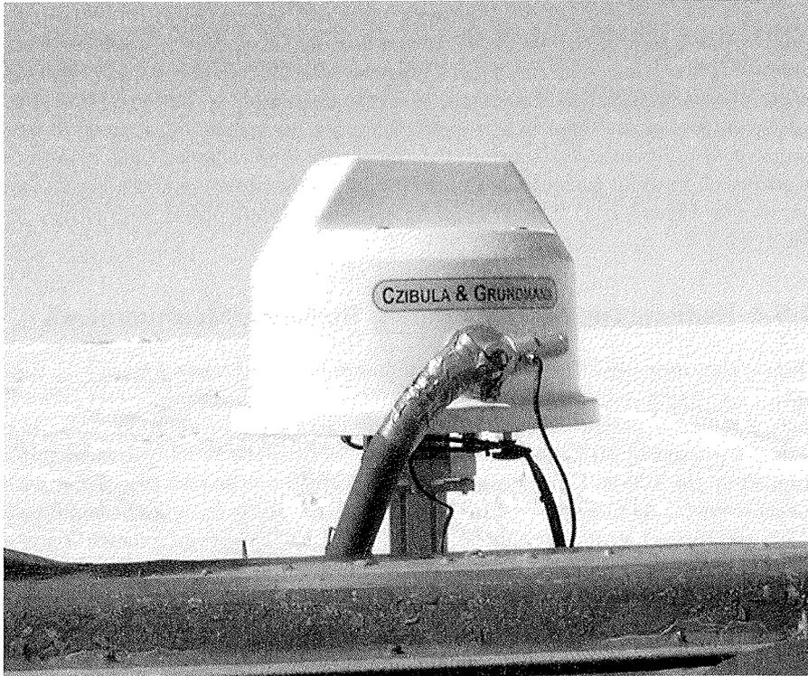
Figure 4.11: Skyscanner with the optical fibre attached for radiance measurements. Currently the entrance optics points near the horizon opposite the position of the sun. The optical fibre is protected by a flexible heated insulated tube.
